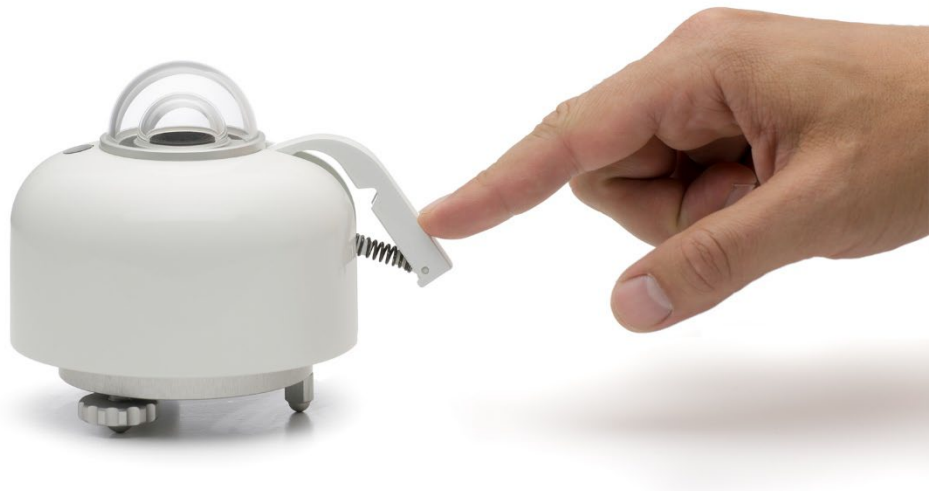
Figure 4.2.2 Installation of sun[e]'s sun screen
